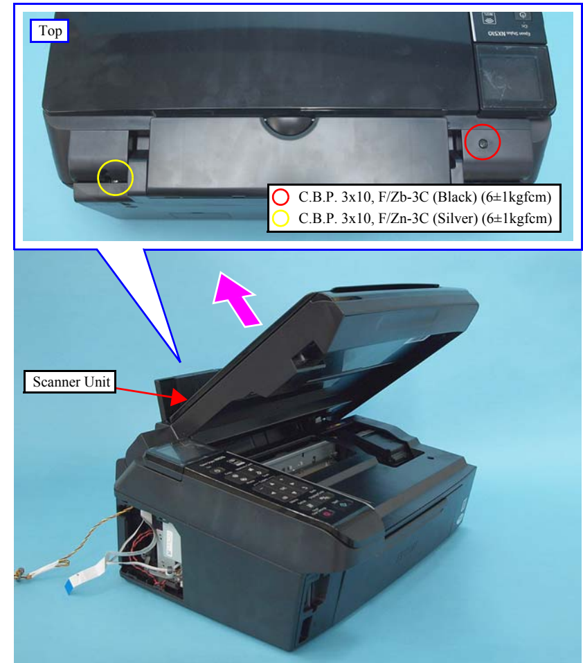
Figure 4-9. Removing the Scanner Unit (3)
